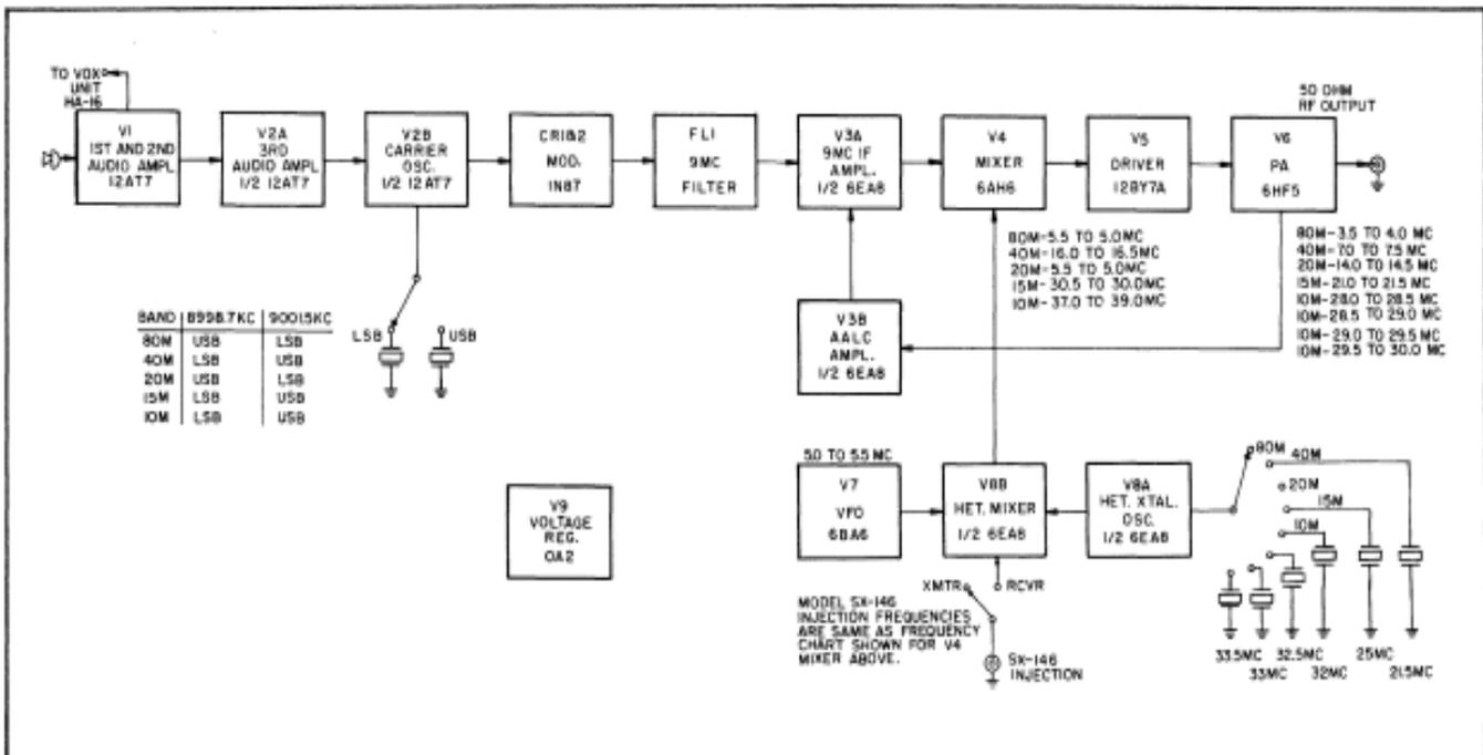
Figure 6. Block Diagram of Model HT-46 Transmitter.
