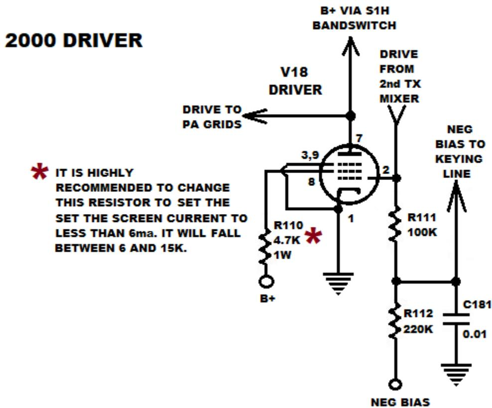
The goal, when adjusting the value of R110, the screen resistor is, to get the screen current below 6ma and the screen voltage below 190vdc. For first run calculations use 190vdc and 0.005ma. in the chart below. The calculation will get close, but differences in tube characteristics will cause variations. The B+ measurement is taken in transmit mode with the transmitter tuned to max power out.
