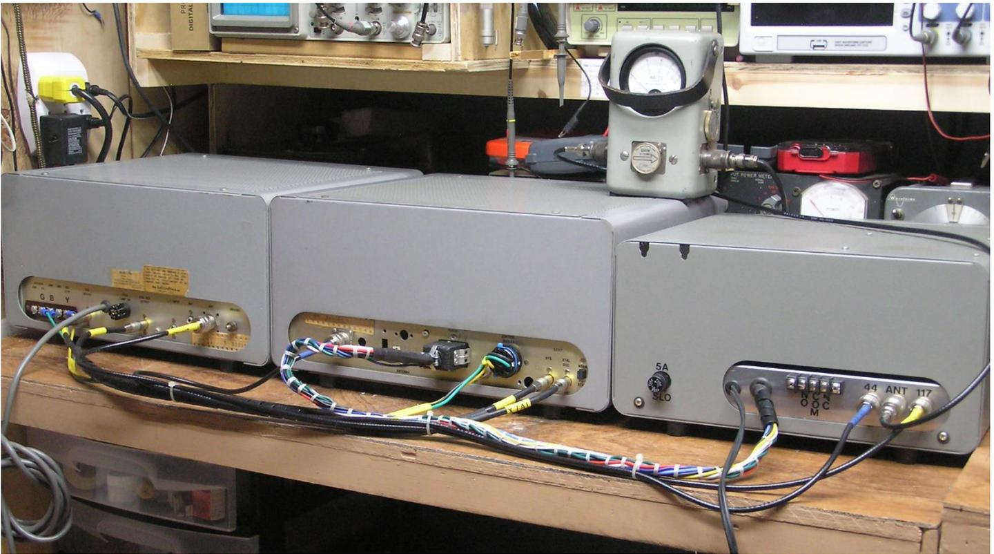
I used a good quality soldered RCA plugs, with stain relief, to make the two oscillator patch cords. The coax patch cords are marked with shrink tubing labels. Thanks to W5IO for the RG62 and a couple tubes.
