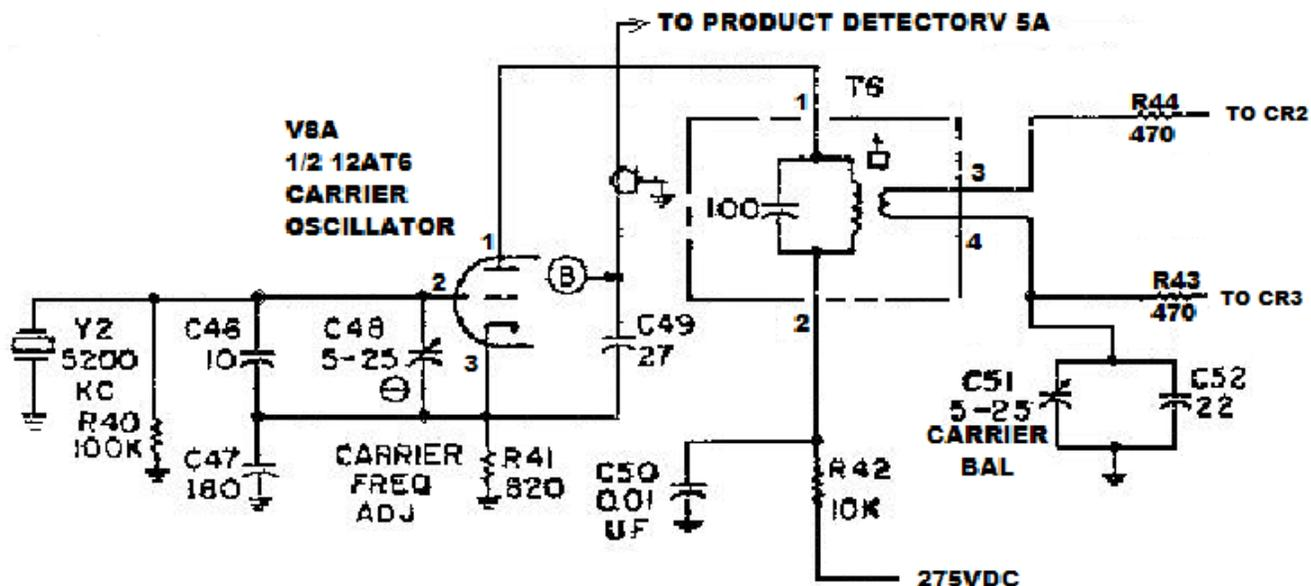
Connect a 10x scope probe to test point B (top of C49 connected to pin 3 of V8A). The other end of the scope probe will be alternately connected to a scope or a frequency counter.
