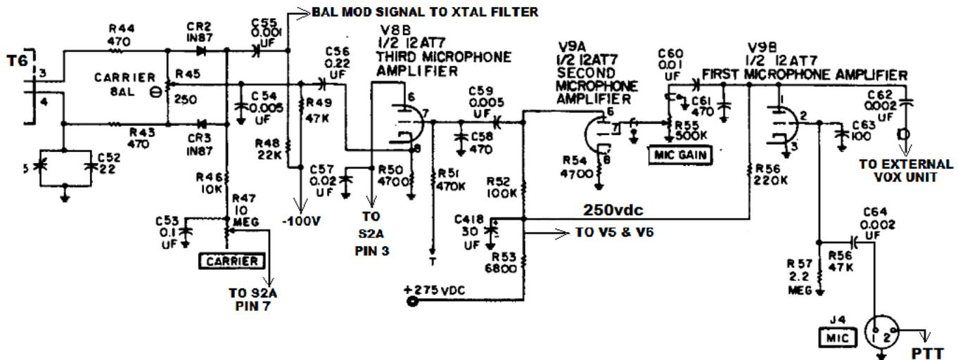
Read the following procedure and follow the flow on the schematic once or twice before you start analyzing the ckt performance.
