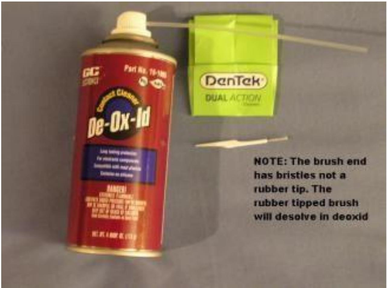
**NOTE: The brush end has bristles not a rubber tip. The rubber tipped brush will desolve in deoxid**
