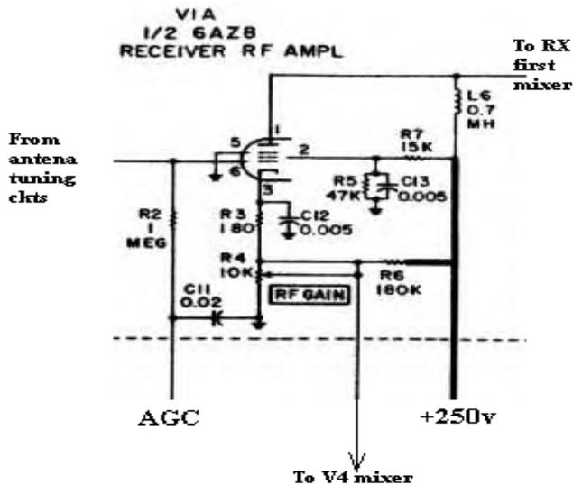
Note the RF GAIN control also controls the gain of the second RX mixer V4.
