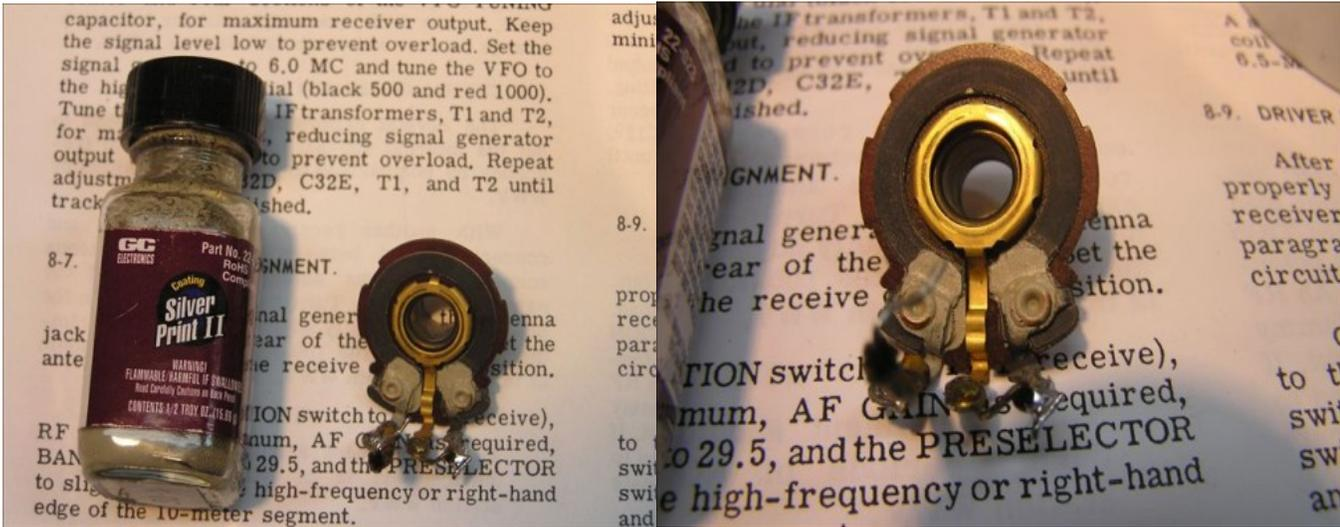
I believe the construction of the pot precludes any of the controls from reaching ideal 0 ohms and that the vast majority of rigs would benefit from some type of corrective action.
