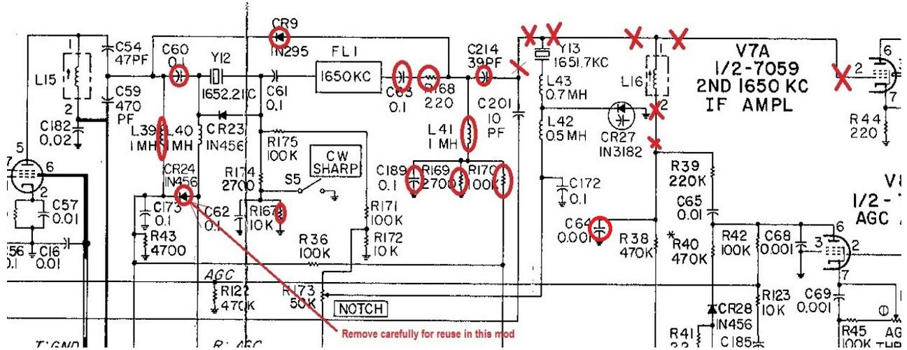
When disconnecting wires and components from L16 note which pins are 1 and 2. The other pins (3 & 4) of L16 are not internally connected and can be used as tie points for adding components. Very handy....
