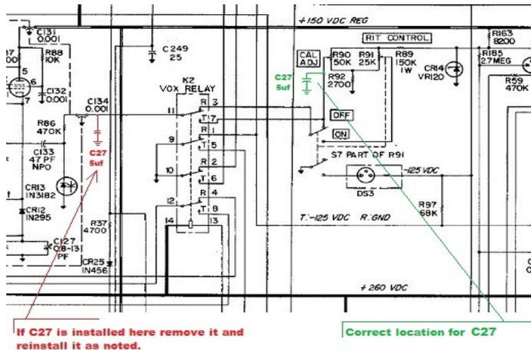
The existence of and placement of C27 although not a part of the upgrade should be noted. There is a chirp and or FM problem in all the SR series radios. C27 eliminates the problem unfortunately it was installed in the wrong place. NOTE the drawing above.
